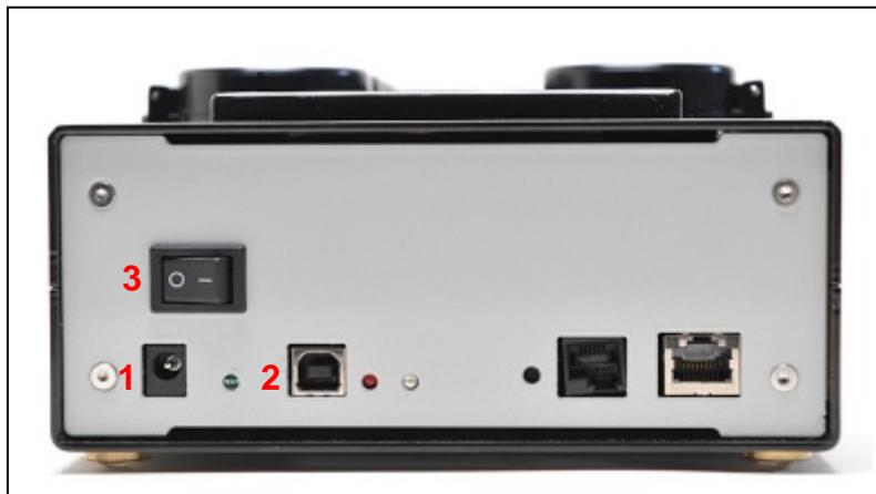
Fig. 1. RVLM – Front panel: (1) Power connector, (2) USB Connector, (3) Power switch
