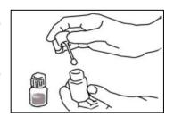
**Note:** do not re-insert the swab into the vial containing the neutralizing solution.
