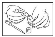
**Note:** the vial grow in 2 liquid phases: the upper one consisting of white oil transparent (does not change during the analysis), formed at the bottom of the vial from the water with which the reagent is dissolved. The color of the second phase will develop fully within 15-20 minutes from the dissolution of the reagent and that is what must be observed for the evaluation of the results of the analysis.
